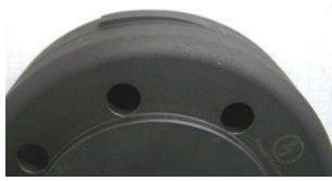
Have a look at the new rotor. You will find on its circumference 2 protrusions (noses). They serve for impulse. The moment the elevation reaches the sensor, it triggers the spark. Do not forget that your Yamaha engine turns anticlockwise (seen onto the face of the rotor).
