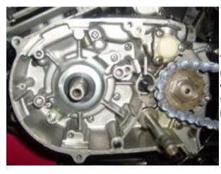
Take the woodruff key from the crank pin. It will not be needed anymore and prevent assembly. If you forget this right at start, you will have to take the whole new unit off again to get access to the key.
