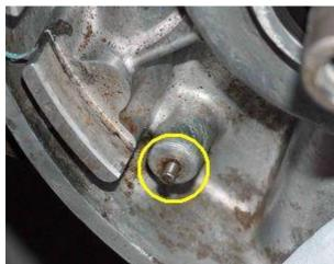
Check whether there is still a small dowel at the circumference of the dynamo seat. This is part of the old dynamo arrangement preventing the customer from installing the original unit wrong side up.
