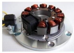
The stator assembly consists of 2 consecutive layers of adapting plates.
