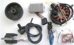
Magnet based generator with integrated ignition. Output at 12V/150W DC. Solid state ignition with own power supply from within the system. Replaces old dynamo, regulator and ignition coils.
