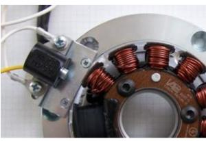
Please note that the rectangular holder plate for the pickup module is only loosely fixed to the base plate with the 2 small countersunk screws M3, as you will have to take off the right screw and shift the sensorplate a little to the side to gain access to a screw hole for assembly. As this small screw is volatile, be careful when tightening (we add 2 extra).
