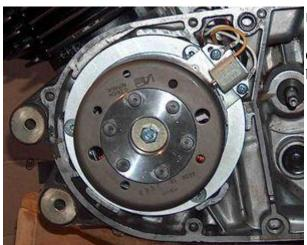
Put the rotor on but do not tighten it yet.
