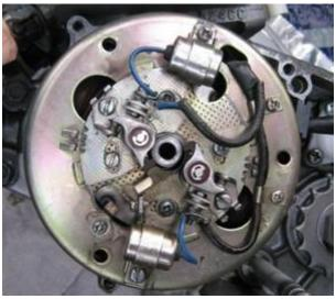
Disconnect all wires to the old dynamo, regulator and ignition coils and take those parts off.
