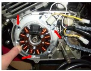
Place the base onto the engine and fasten loosely with the bottom 2 countersunk screws.
